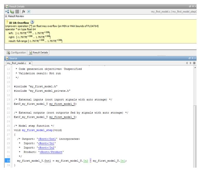
This orange check shows a potential overflow issue when multiplying the signals from the inports In1 and In2. To fix this issue, you must return to the model.
