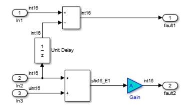
You can avoid the **Overflow** in several ways. One way is to constrain the value of the signal in\_battery\_info that is fed to the Sum block. To constrain the signal:
